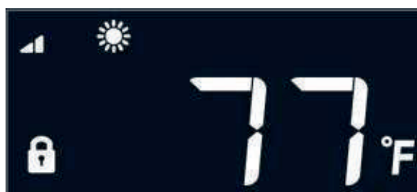
Heating in smart mode main interface
