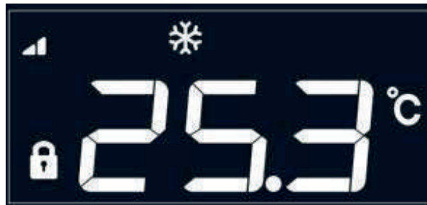
Cooling in smart mode main interface
